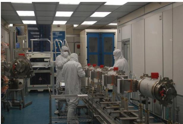
Figure 3: Cavity String Assembly.
