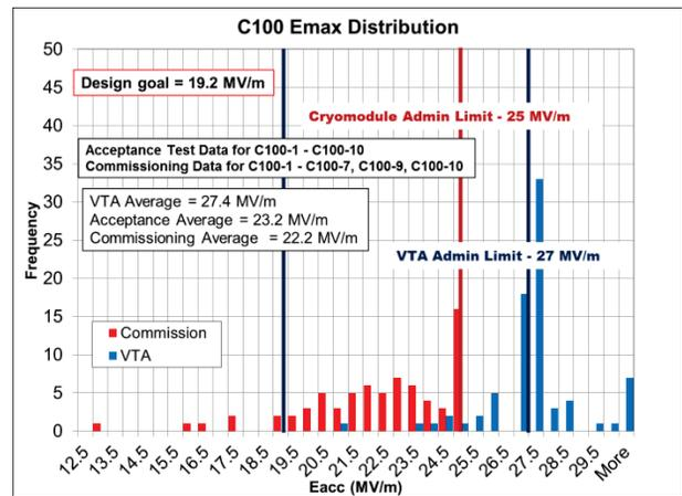
Figure 5: Emax Distribution for VTA and Commissioning .
