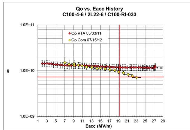
Figure 11: Typical  $Q_0$  Curve VTA and Commissioning.
