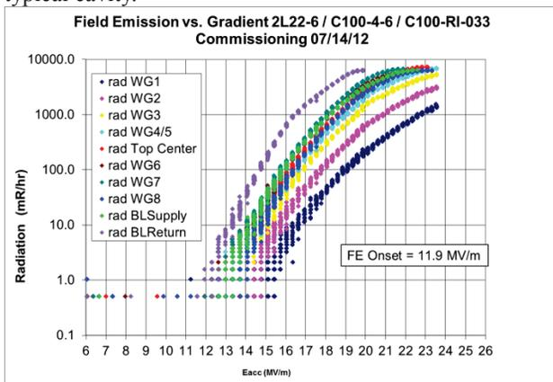
Figure 7: Plot of X- Ray Production for a Typical Cavity.
