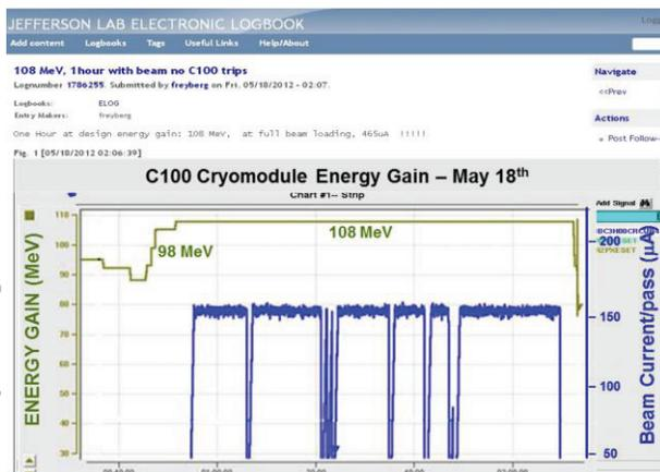
Figure 15: Extended Run at 108 MV and 465  $\mu$ A.
