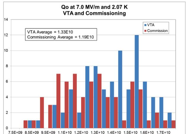
Figure 12:  $Q_0$  Distribution at 7 MV/m.
