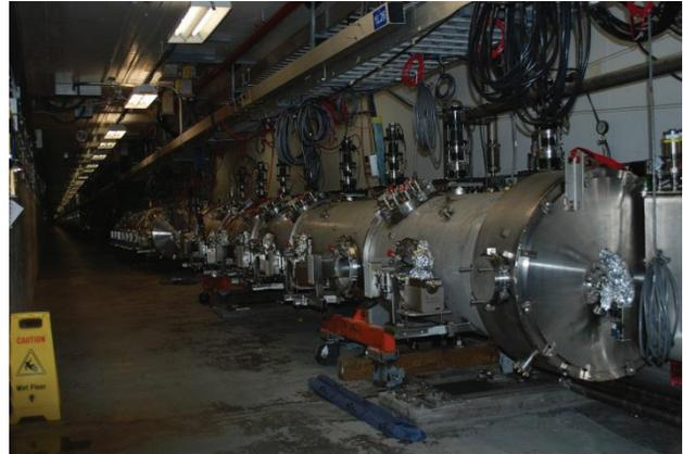
Figure 4: C100 cryomodule in the Tunnel.
