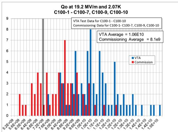
Figure 10: Distribution Q0's at 19.2 MV/m.
