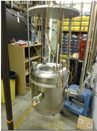
Figure 5: \beta=0.53 HWR mounted on insert in preparation for a “dunk” test. The cavity vacuum space is actively pumped during cooldown and testing.
