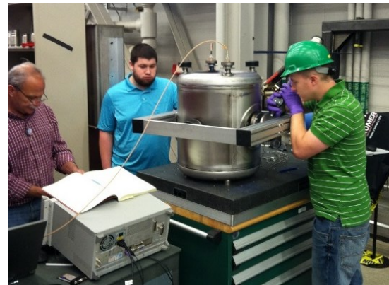
Figure 2: Tuning sensitivity and stiffness measurements being performed on the \beta=0.53 HWR.
