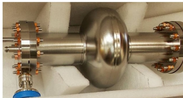
Figure 1: First laser welded 1.3 GHz SCRF cavity.
