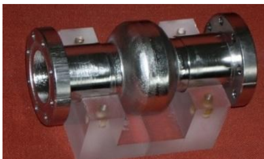
Figure 6: 1 st Laser welded 3.9 GHz SCRF cavity.
