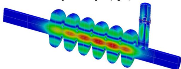
Figure 5: HFSS model used to estimate the QL of HOMs showing the 1506.48 MHz mode of the  $\beta=0.67$  cavity.
