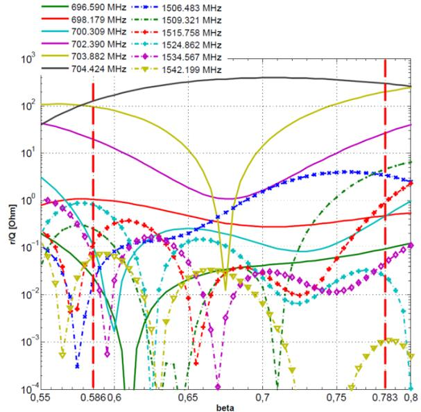
Figure 4:  $r/Q$  with respect to the proton  $\beta=v/c$  for fundamental and first longitudinal HOM passbands.
