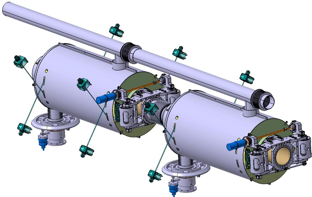
Figure 7: Arrangement of a pair of cavities in the 4-cavity string showing the bottom position of the power coupler, cold tuning system, inter-cavity bellow, TA6V tie-rods which are part of the cavity supporting systems, magnetic shields and two-phase cryogenic pipe connected to the top of the helium vessels.
