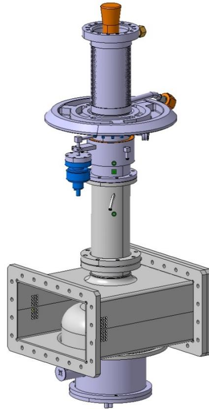
Figure 10: Model of the fundamental power coupler.
