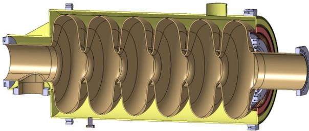
Figure 3: 6-cell  $\beta=0.67$  cavity 3D model.
