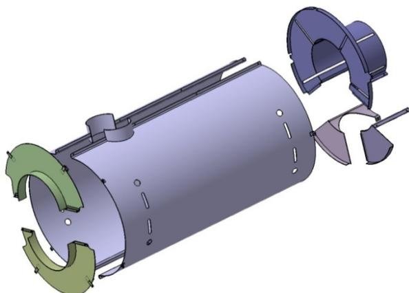
Figure 8: Elements of the magnetic shield.
