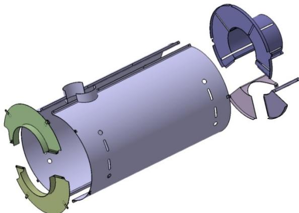
Figure 8: Elements of the magnetic shield.
