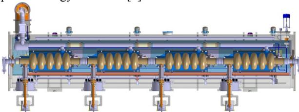
Figure 1: Cut view of the high beta cryomodule.
