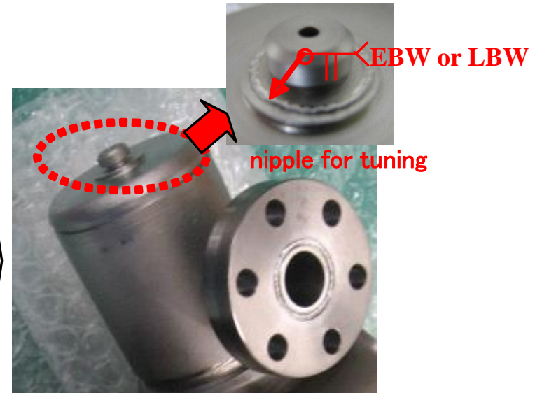
EBW for nipple, port and inner conductor
