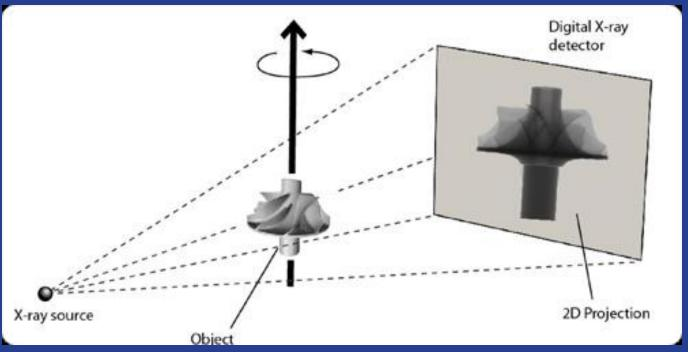
The X-ray tube (open or sealed) produces a conic beam of electron that penetrates the object to be analyzed, and a digital signal is interpreted by the 2D detector as a Digital Radiograph image.
