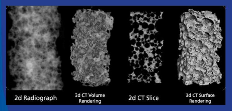
From a series of 2D Radiographs and after calibration, the CT reconstruction software provides 3D volume results using Filtered Back-Projection algorithm (Feldkamp). 3D CT data are rendered as voxels (volume element) with threedimensional resolution from a few micrometers (microCT) to hundreds of micrometers depending on X-ray detector pixel size.
