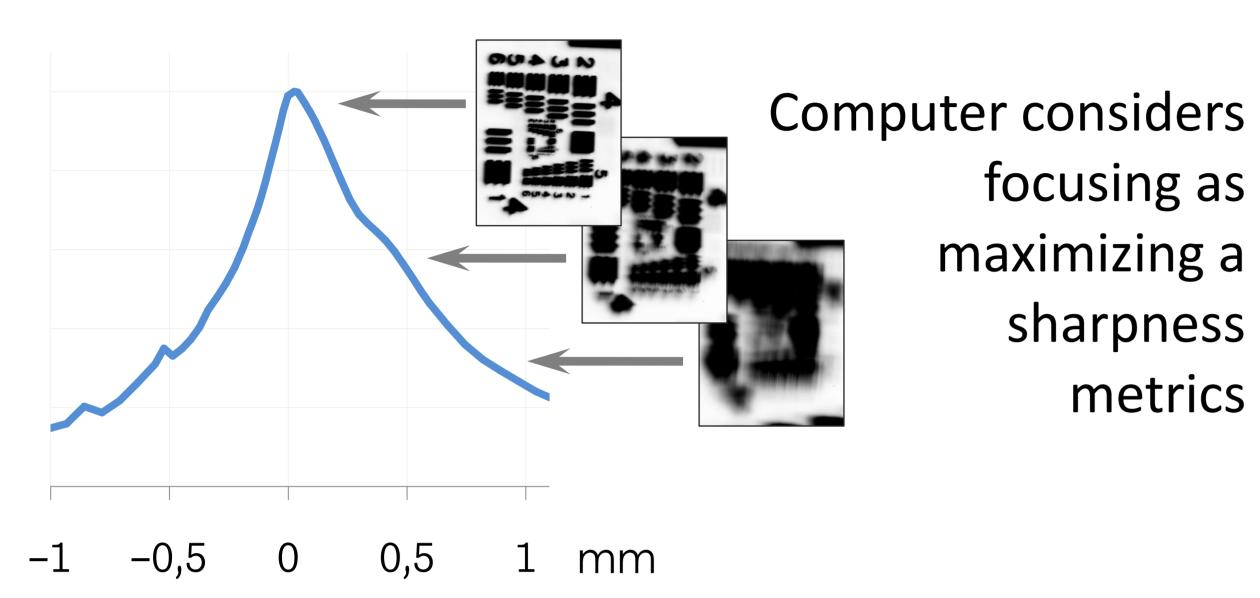
An algorithm changes camerasurface distance until the metrics peak is reached
