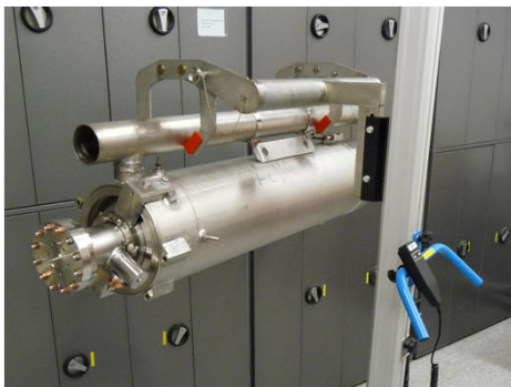
Figure 2. Cavity lifter with cavity in helium tank
