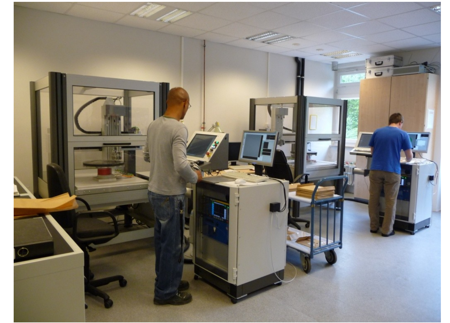
Equipment for eddy current scanning of XFEL niobium at DESY
