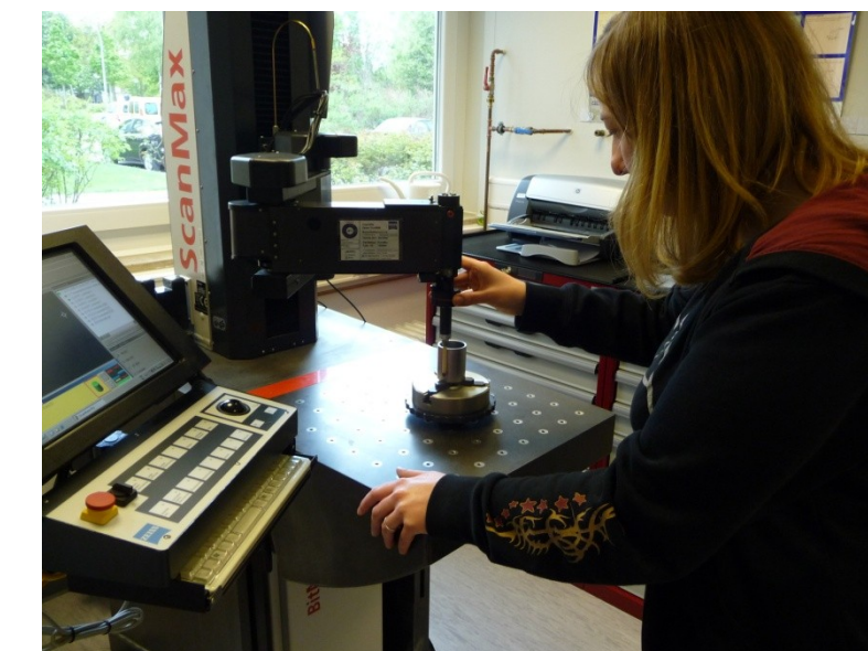
Equipment for tactile 3D dimension measurement
