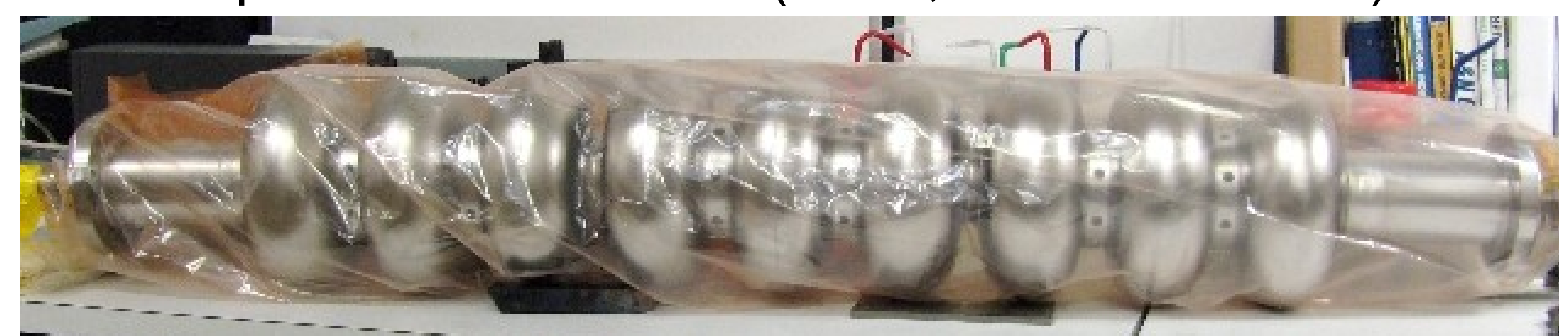
9-cell cavity hydroformed at DESY from Black Lab. tubes completed at JLAB
