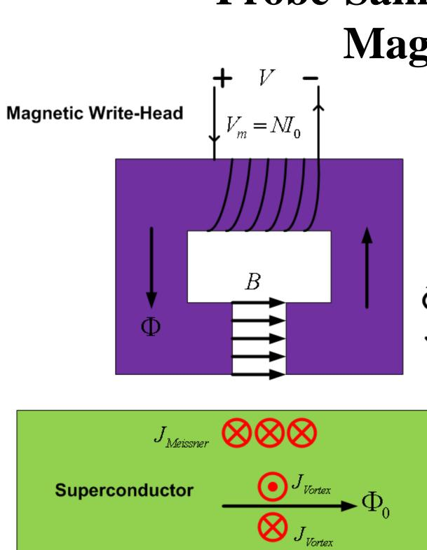
$$\begin{cases} V = \frac{d\Phi}{dt} \\ \Phi = \frac{V_m}{R_{eq}} \implies V = \frac{d}{dt} \left(\frac{NI}{R_{eq}}\right) = \frac{N}{R_{eq}} \end{cases}$$
