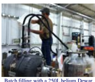
Batch filling with a 250L helium Dewar
