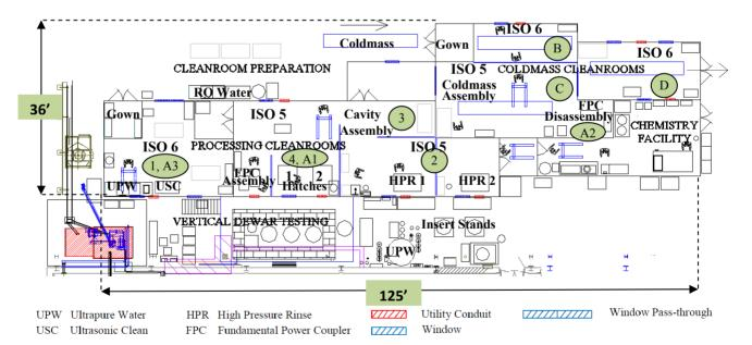
Figure 1. Proposed cleanroom layout for cavity processing and coldmass assembly.
