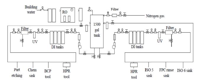
Figure 2. Sketch of a proposed ultra pure water system.
