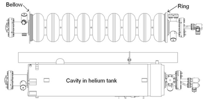
Figure 3: Sketch of cavity with ring and bellow (above); Cavity in helium tank (below).
