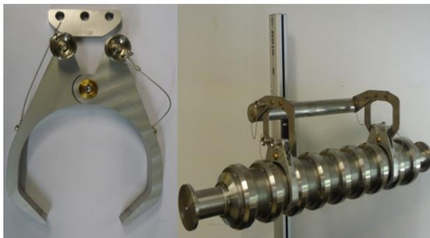
Figure 9: Gripper and cavity lifter carrying a dummy cavity for calibration.
