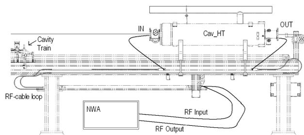
Figure 10: Sketch of new RF-cabling for cavity in helium tank.
