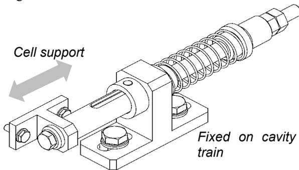
Figure 2: Sketch of centering unit for cavity on the train.
