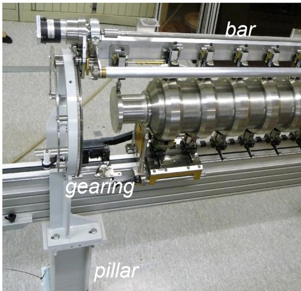
Figure 6: New design of gearing, drive chassis and measurement bar supported by the steel pillar.
