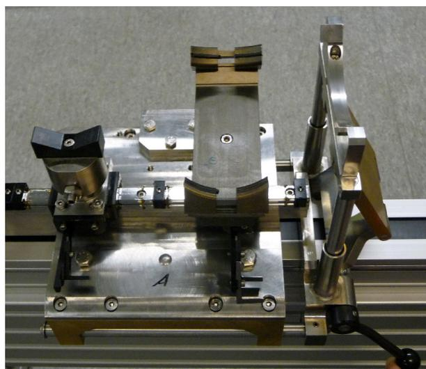
Figure 5: Heavy duty lift unit seen on the right side. It is manually operated.
