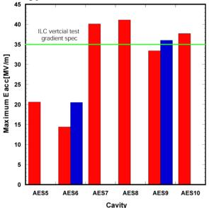
Figure 2: Gradient performance of 9-cell cavities from the second AES production batch.
