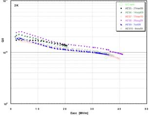
Figure 4: Q(Eacc) curves of 9-cell cavities from the second production batch by AES. 4 out of 6 exceed the ILC vertical test gradient and  $Q_0$  specification.
