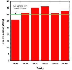
Figure 7: Best gradient performance of 9-cell cavities from the second AES production batch. AES5 and AES6 were improved by mechanical polishing for removal of known defects.
