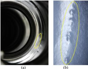
Figure 6: (a) Surface depression at a radius close to that of the stiffening ring (circled by ellipse). (b) Surface damage in the depressed region after the cavity was exited to a gradient of > 30 MV/m.
