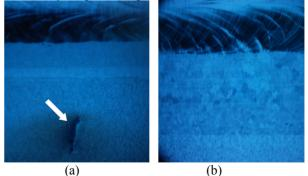
Figure 5: (a) Weld splatter (arrow) observed on the inner cavity surface near the equator electron beam weld in an as-received cavity. (b) Clean surface with effective weld splatter removal by using a light BCP etching prior to the heavy EP processing.
