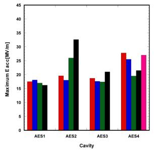
Figure 1: Gradient performance of 9-cell ILC cavities from the first AES production batch.
