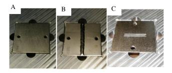
Figure 1: Samples are fabricated from high RRR niobium, 2" x 2" x 0.079"; A: As-received sample, B: Welded (full penetration) sample, C: Scratched samples.
