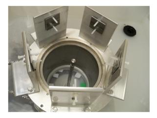
Figure 2: High-pressure rinsing of niobium samples; 5 samples on tool per run  $(5.25 \text{ sec/in}^2)$
