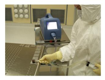
Figure 3: A QIII+SPD surface particle counter will be used to measure particles on samples before and after processing.
