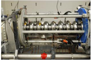
Figure 1: Cavity outer surface water irrigation setup added to the JLab EP machine. An array of nozzles spray chilled water at selected iris and/or equator regions.
