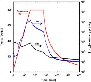
Figure 2: Standard ILC cavity vacuum furnace heat treatment temperature profile. The partial pressure of  $H_2$  and  $H_2O$  of a typical 9-cell heavy-electropolished cavity is also shown.
