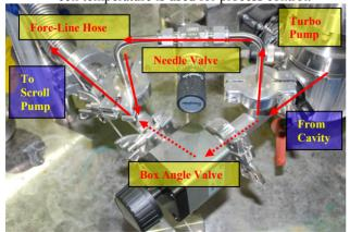
Figure 3: A slow pump down unit permanently installed in the test stand between the turbo pump and the fore-line vacuum hose. During initial pump down, a highimpedance line is formed by closing the box angle valve and slightly opening the needle valve.
