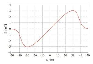
Figure 7: Magnetic field along the beam axis.
