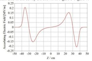
Figure 5:  $E_z$  along the beam axis.
