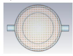
Figure 3: Magnetic field of the fundamental mode in the top view.
