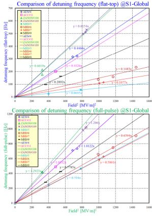
Figure 13: Correlation between the detuning frequency and the square of the field for rise-up, flat-top and fullpulse including the linear fitting.
