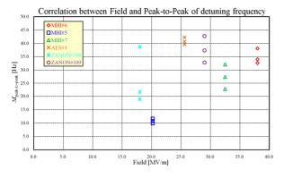
Figure 18: The correlation between the excursion peak-topeak of the detuning frequency at flat-top and field. The best three results are shown here.
