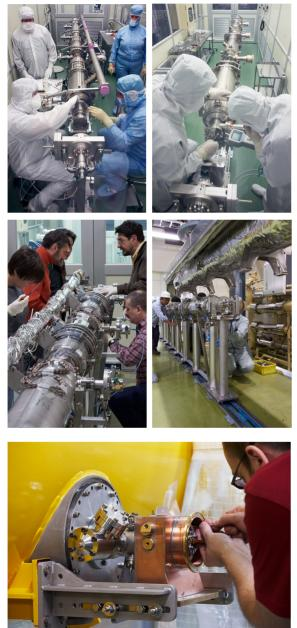
Figure 5: Assembly work of the cryomodules in progress.
