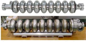
Figure 1: TESLA-type (top) and TESLA-like (bottom) cavities.
