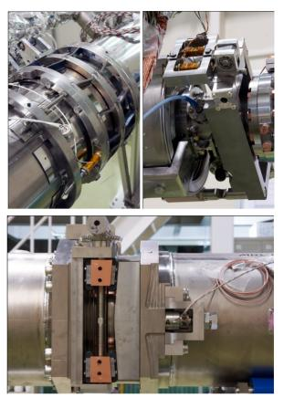
Figure 3: Blade (top-left), Saclay (top-right) and Slidejack (bottom) tuners.
