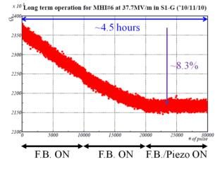
Figure 19: The trend of  $Q_L$  during the long term operation for MHI-06.
