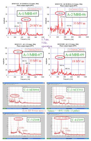
Figure 9: The result of the mechanical vibration modes measured at high power for Cryomodule-A, and at low power for Cryomodule-C.
