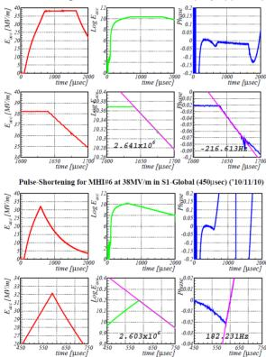
Figure 11: The examples of the linear fitting range for the pulse width of 1500 µs (top) and 450 µs (bottom). The red graph shows the accelerating gradient, green shows the logarithmic gradient, blue shows the phase for MHI-06, and purple line shows the fitting line.
