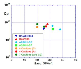
Figure 24: The results of the dynamic loss measurement. The measurements on 26/Nov. and 30/Nov. were carried out with the detuned cavities. Every  $Q_0$  value was below  $10^{10}$ .
