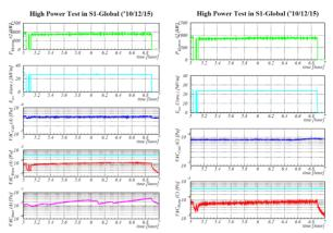
Figure 23: The trend of helium level, helium pressure, helium flow and vacuum during the long term operation (17:00-19:00). 12:00-19:00 (top-left) and 17:00-19:00 (others). The vacuum level at three locations for Cryomodule-A (left) and two locations for Cryomodule-C (right) are shown in the bottom figures.
