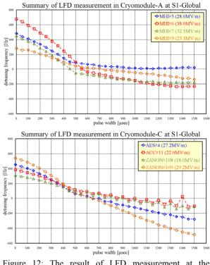
Figure 12: The result of LFD measurement at the maximum gradient for every cavity.
