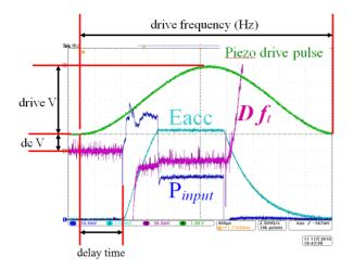
Figure 16: One pulse of sine curve added to piezo for the compensation of LFD. The blue shows the input power, light blue shows the accelerating gradient, purple shows the cavity phase and green shows the drive pulse to a piezo. Four adjustable parameters exist, that is, drive frequency, pulse height, pulse offset and delay time for the piezo drive.
