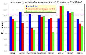
Figure 8: The achieved gradient values for eight cavities in vertical and cryomodule tests. The maximum average gradient is 30.0 MV/m at vertical test, 27.7 MV/m for single cavity operation and 26.0 MV/m for simultaneous operation of seven cavities at cryomodule test. The purple dotted line shows 31.5 MV/m of the ILC specification.
