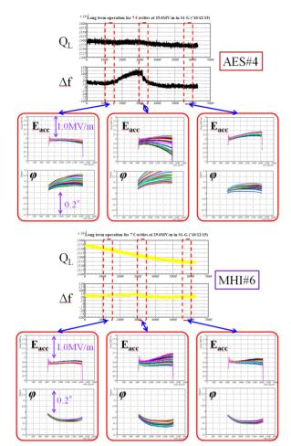
Figure 22: The superimposed RF pulses at the flat-top for three periods during the long term operation.
