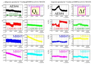
Figure 20: The trend of  $Q_L$  and the detuning frequency during the long term operation for 7 cavities.
