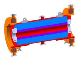
Figure 4: Sectional view of the Solenoid layout with moveable compensation-coils.
