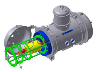
Figure 2: The cryostat of the cw-LINAC Demonstrator with the supporting frame (green) and the CH-cavity (yellow) in its centre embedded by two sc solenoids (redorange).
