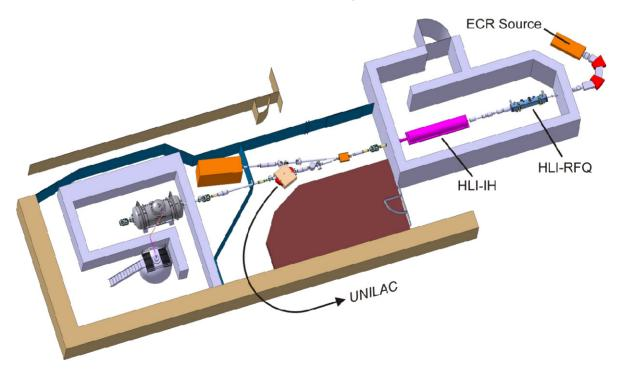
Figure 1: The future layout of the GSI accelerator facility with the cw-LINAC Demonstrator integrated in the existing High Charge Injector (HLI).
