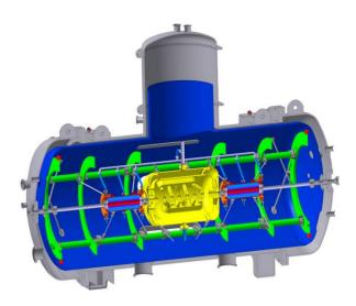
Figure 3: Sectional view of the cryostat. On the top space for a reservoir of liquid helium as well as of liquid nitrogen is reserved.
