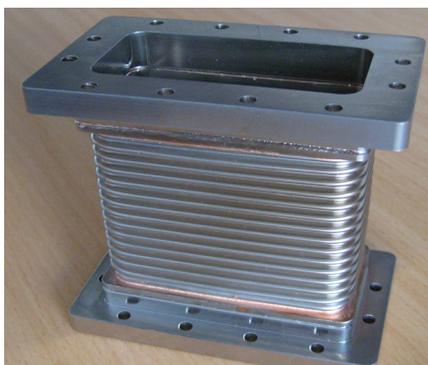
Figure 2: Rectangular stainless steel bellow (100 mm length) as part of the rf waveguide transition (WR 284) for the injector upgrade module (before copper plating).
