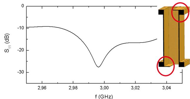
Figure 1: Heat radiation intercept of the RF waveguide at 80 K (schematic layout and RF properties).
