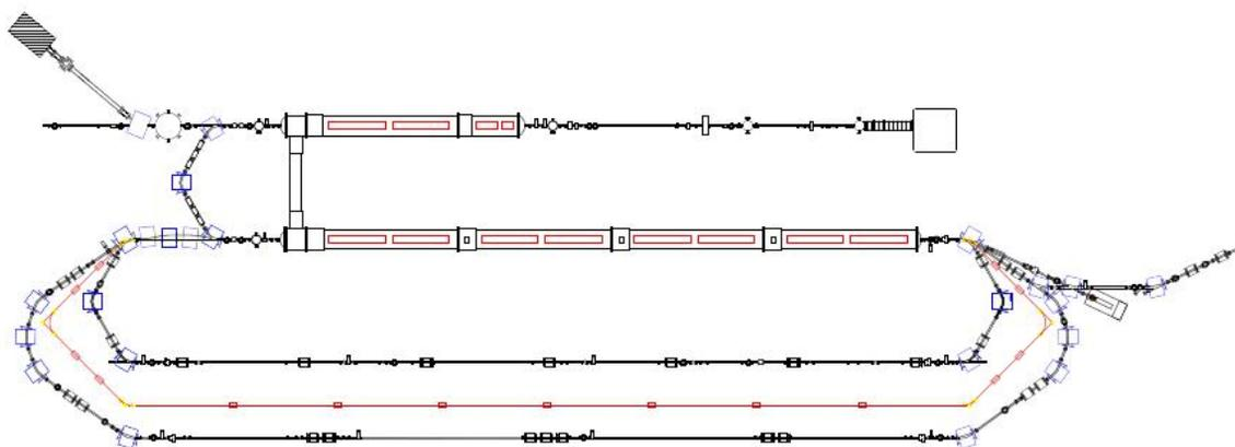
Figure 3: Floor plan of the S-DALINAC indicating the third recirculation to be added: The new recirculation beam line (red) can be placed between the existing ones minimizing the investment cost and the required shut down period.
