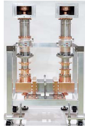
Figure 2: cERL couplers on the coupler test stand
