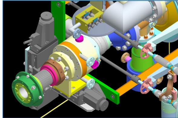
Figure 10: Solenoid with two step motors.
