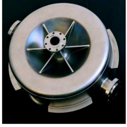
Figure 4: 450 MHz single spoke cavity.
