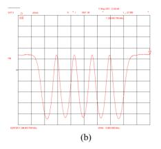
Figure 3: 1.3 GHz 5-cell cavities for high current accelerator. (a) 5-cell cavity (b) field flatness after pre-tuning.
