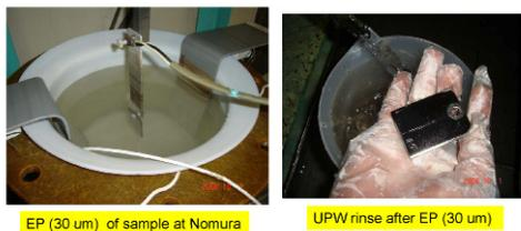
Figure 5: Left-hand side: A picture for the EP process of Nb-plate sample. Right-hand side: A picture for the Ultra-Pure Water (UPR) rinse after each EP process.
