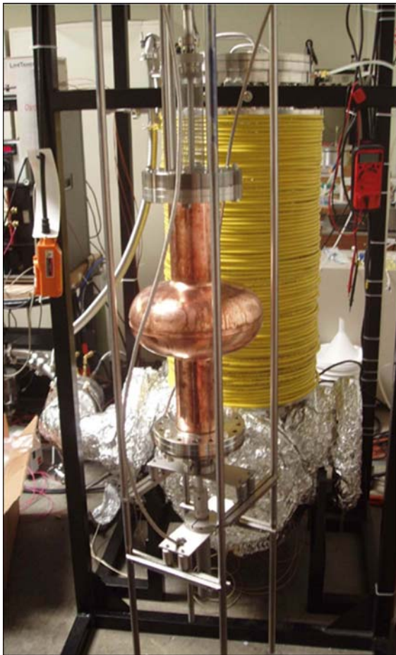
Fig. 2: Photograph of the CED™ system, showing a 2.2 GHz copper RF cavity for scale.
