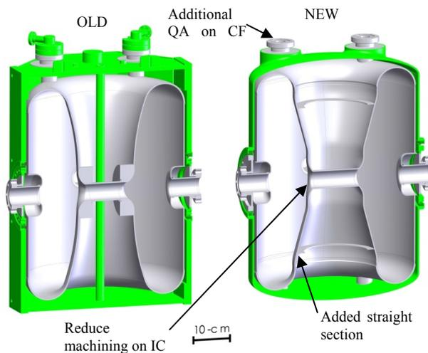
Figure 2: FRIB half-wave resonator old and new design.
