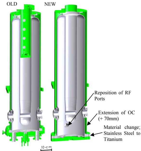
Figure 1: FRIB quarter-wave resonator old and new design.
