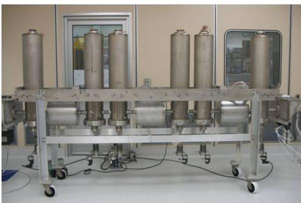
Figure 7: The ReA  $\beta = 0.041$  coldmass assembled in the MSU cleanroom [5]. The ReA  $\beta = 0.041$  cryomodule serves as prototype cryomodule for FRIB.
