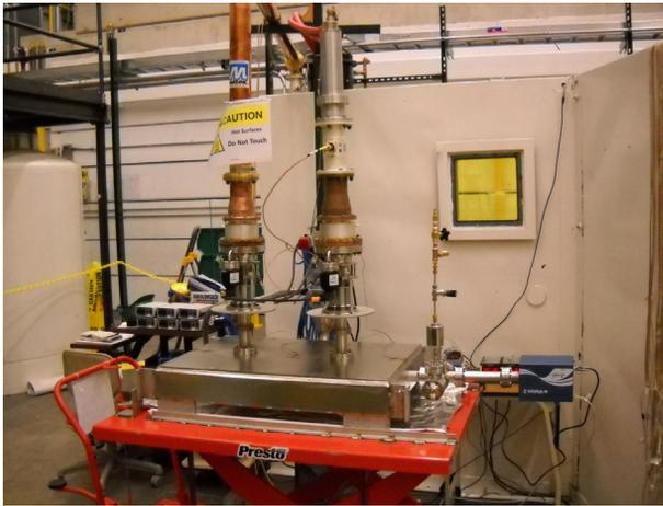
Figure 8: Vacuum baking and RF conditioning teststand for the FRIB HWR power couplers.
