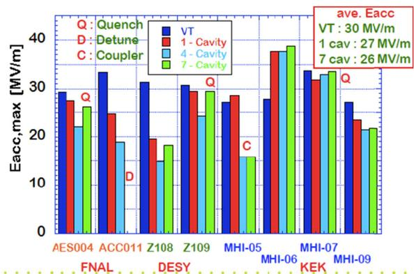
Figure 7: (top) S1-global cryomodule installed at STF, and (bottom) the gradient distribution in cavity-string operation (right three) compared with the result from their individual vertical test (most left) [24, 27, 28].
