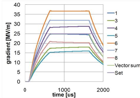
Figure 8: LLRF control to compensate the Lorentz force detuning, and the vector sum stability in S1-Global cavity-string test.
