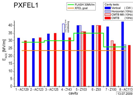
Figure 5: (top) Prototype XFEL cryomodule at FLASH, and (bottom) field gradient distribution [22].
