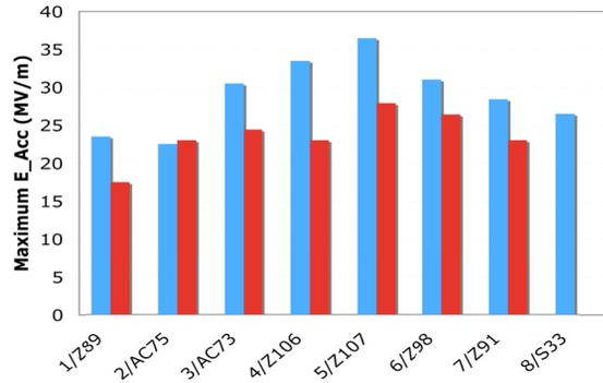
Figure 6: (top) Cromodule-1 at NML, and (bottom) the field gradient distribution (right) compared with individual test in horizontal position (left) [23].
