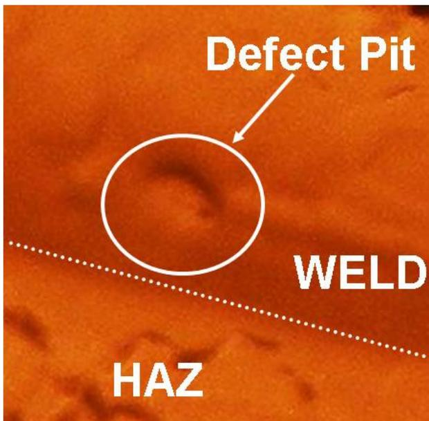
Figure 2: The 9-cell reentrant cavity pit defect.
