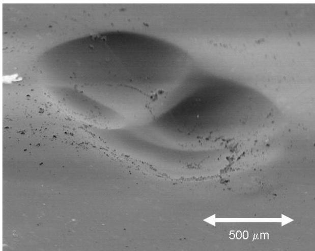
Figure 3: Pit defect found at quench location in a single cell cavity. The bar is 500 microns.
