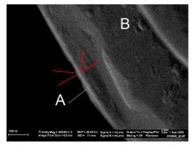
Figure 6. SEM image of a breaking edge of a TiN coated sample. The red marked area indicates the layer.
