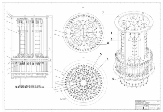
Figure 2: Detailed CAD drawing of inner assembly. 1: outer Ti wire, 2: coupler ceramics, 3: current supply, 4: Ti wire for front side coating, 5: front side ceramics, 6: isolation, 7: support frame.
