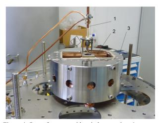
Figure 4: Setup for waveguide window coating. 1: current supply, 2: ceramic, Ti wire inside the pillbox is not visible.
