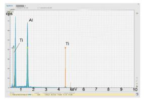
Figure 5. EDX spectrum of a TiN coated sample
