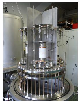
Figure 3: Inner assembly, with 4 mounted ceramics. 1: flexible suspension of the wire, 2: ceramic, 3: vessel flange.
