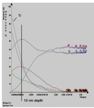
Figure 8. Depth Profile taken with GDOES
