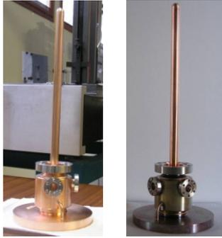
Figure 15: SS-03 power coupler before (left) and after (right) RF conditioning up to 7 kW CW and the break of the window.
