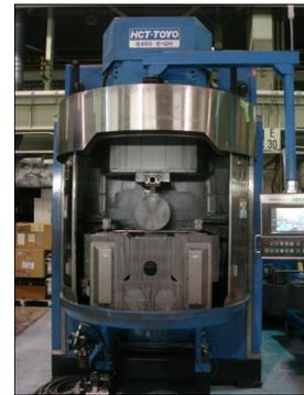
Figure 4: A slicing machine for silicon wafer, which we used for niobium ingot.
