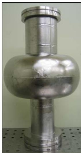
Figure 8: A LL end single cell cavity made of the sliced niobium sheets (1300MHz).
