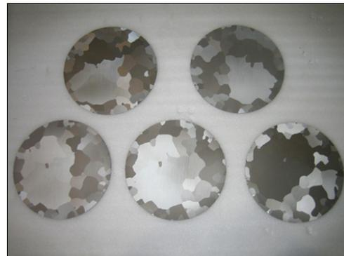
Figure 6: Successfully sliced niobium sheets from Tokyo Denkai.
