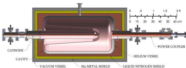
Figure 7: 112 MHz – quarter wave BNL SRF gun cavity string. *Courtesy A. Burrill.*
