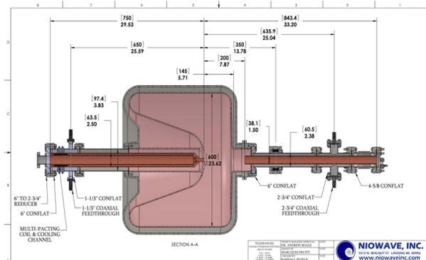
Figure 6: 200 MHz – quarter wave Wisconsin University SRF gun cavity string. *Courtesy NIOWAVE Inc.*
