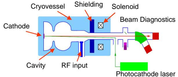
Figure 3: Generic design of the 1.3 GHz – 1.6 cell BERLinPro SRF gun. Courtesy Thorsten Kamps.
