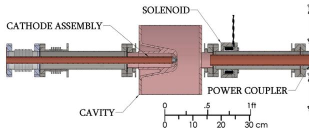
Figure 5: 500 MHz – quarter wave NPS SRF gun cavity string. *Courtesy NIOWAVE Inc.*
