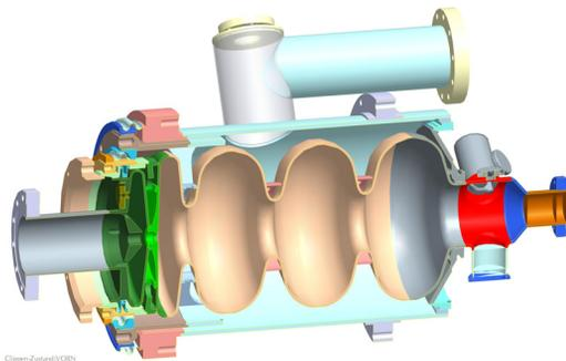
Figure 1: 1.3 GHz - 3.5 cell TESLA shaped FZD cavity.
