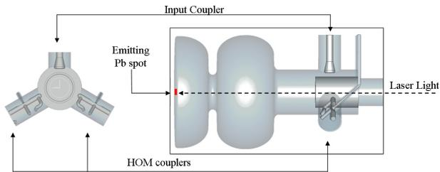
Figure 8: 1.3 GHz – 1.6 cell Pb/Nb hybrid SRF gun cavity. *Courtesy J. Sekutowicz.*
