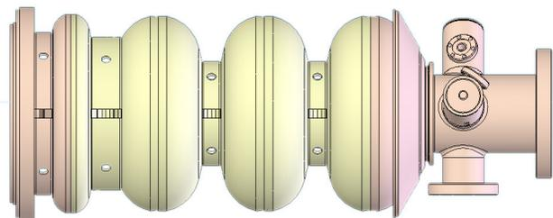
Figure 4: 1.3 GHz – 3.5 cell IHIP SRF gun cavity. Courtesy IHIP PU.
