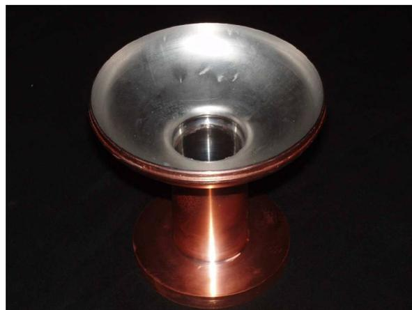
Figure 9: 2.2 GHz Copper RF cavity half-cell coated with Nb using the CED™ process.
