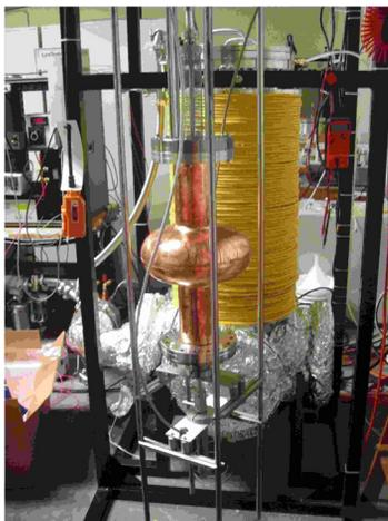
Figure 2: Photograph of the CED<sup>TM</sup> system, showing a 2.2 GHz copper RF cavity for scale.
