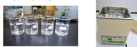
Figure 8: Upper: Various rinsing conditions of the tests. Lower left: Teflon-mesh sheets dipped in various solutions. Lower right: Rinse with ultrasonic vibration.
