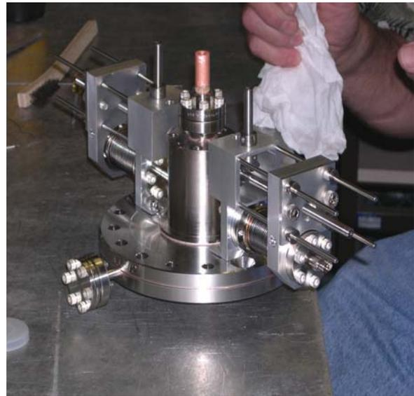
Figure 3.) TE<sub>011</sub> cavity and variable input coupler mechanisms.
