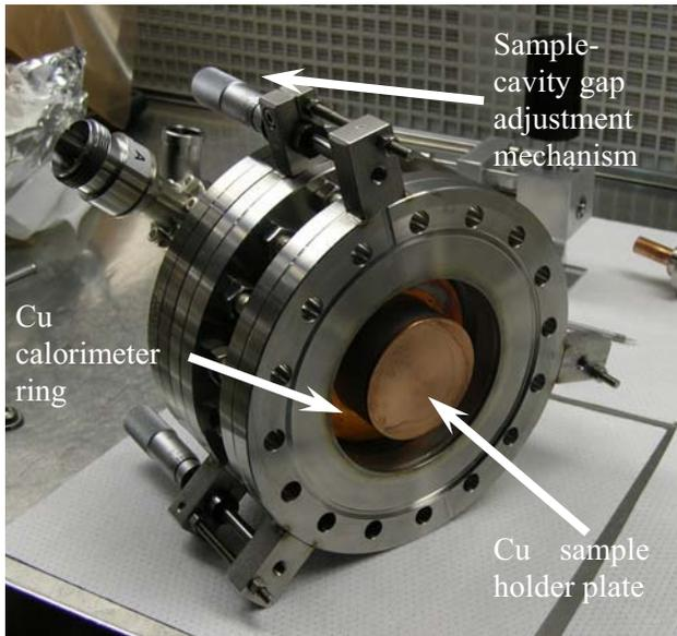
Figure 5.) Sample holder plate showing gap adjustment mechanism and Cu calorimeter ring.
