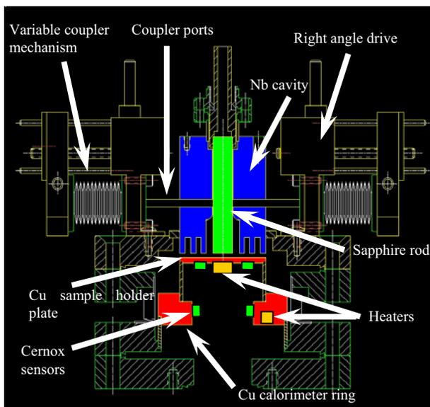
Figure 2.) Schematic of TE<sub>011</sub> cavity and variable input coupler mechanisms.
