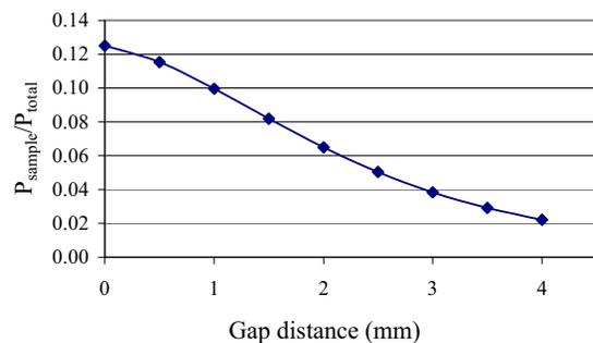
Figure 4.) The plot above gives the fraction of RF power dissipated in the SC sample, as a function of distance between sample and cavity, for fixed field.
