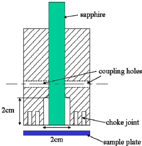
Figure 1.) Schematic of the TE<sub>011</sub> cavity geometry.
