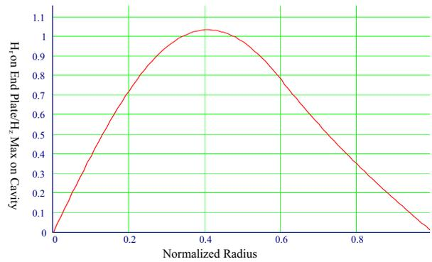
Figure 6.) Radial magnetic field (scaled by the maximum magnetic field of the cavity), whose integral over the sample surface gives the total power dissipated.
