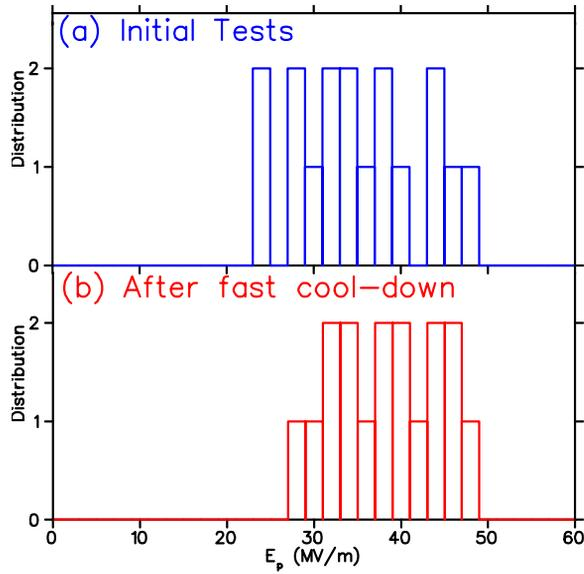
Figure 2: Histogram summarizing cavity performance for seventeen tested cavities. Shown are the numbers of cavities achieving a certain peak surface field at 7W helium load. Initial tests are shown in the top plot and recent status is shown in the bottom plot after testing poorer cavities with a fast cooldown.
