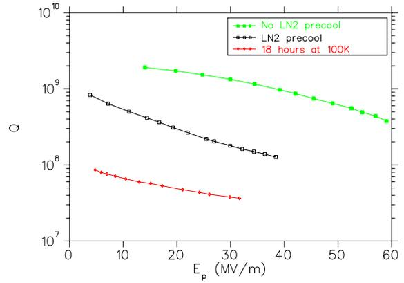
Figure 3: Summary of test results for cavity 17.
