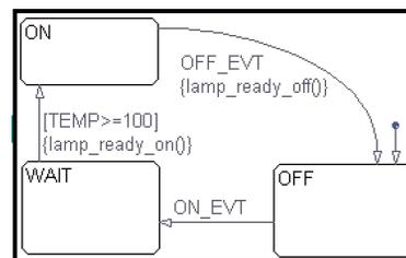
Figure 1: FSM representing a simple water heater
