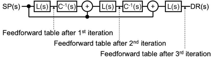
Figure 4: Control theoretical view of a very simple scheme for adaptive feedforward.  $SP(s)$  and  $DR(s)$  shall be the Laplace transforms of the setpoint table of one pulse and the drive that is applied to the cavity (or vector sum).  $P(s)$  is the transfer function of the plant.  $C(s)$  is the transfer function of the controller, which e.g. can be a proportional controller.  $L(s)$  is the transfer function of a closed loop system.
