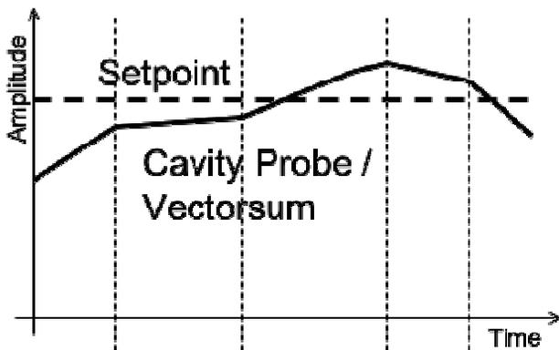
Figure 5: Small part of the flattop of a pulse. The dashed vertical lines define sections, along which an average error  $\Delta x$  and average slope error  $\Delta \dot{x}$  are determined.
