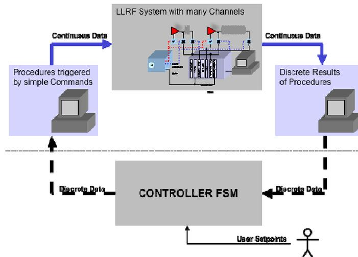
Figure 2: Quantization of LLRF Automation. Seen by the controller FSM, the complex LLRF-System appears as a system with discrete in- and output signals.
