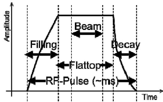
Figure 3: Pulse structure of the accelerating field in a superconducting cavity.
