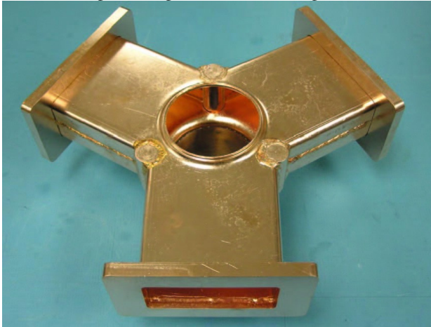
Figure 9. Copper model of waveguide end group.
