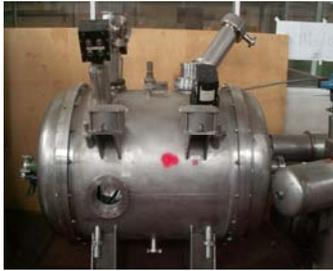
Figure 3: The CM0 module for spoke cavities.
