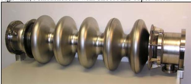
Figure 6. Niobium 5-cell cavity
