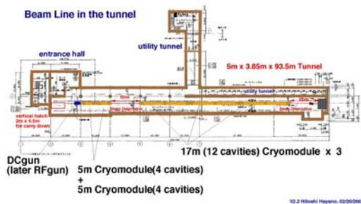
Figure 3 STF tunnel layout plan
