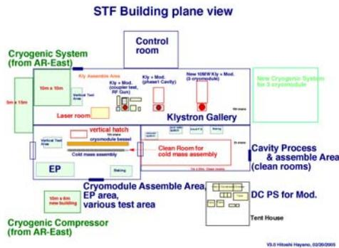
Figure 2 STF plan of building usage
