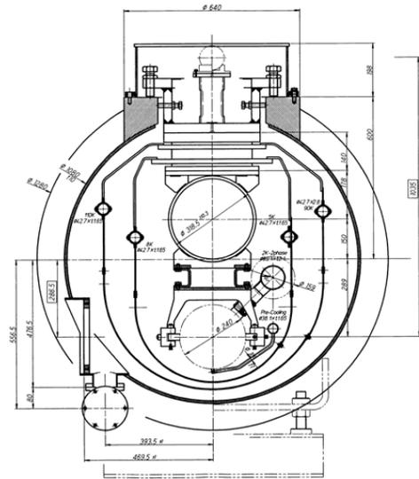
Figure 4 cross-section of STF Phase 1 cryomodule
