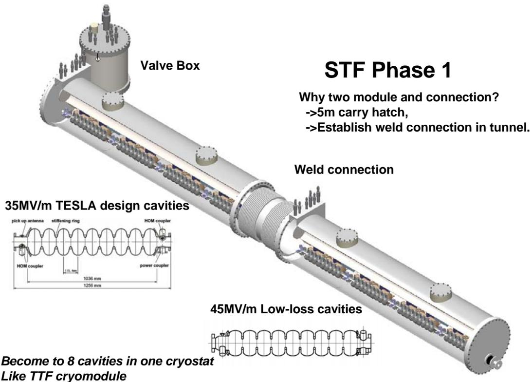
Figure 5 STF phase 1 connected-cryomodule.
