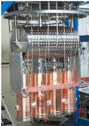
Figure 2: The cold mass of ALPI at INFN/LNL.
