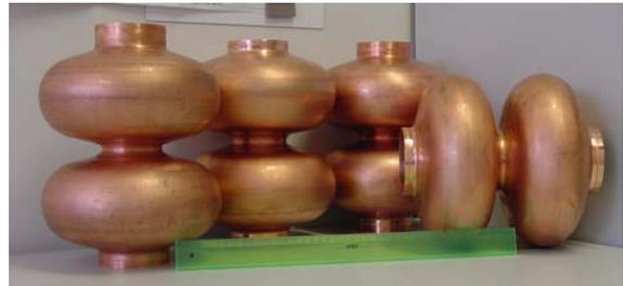
Figure 4: Double cell NbCu clad cavities recently produced at DESY from KEK tubes (no cracks on the inside surface).
