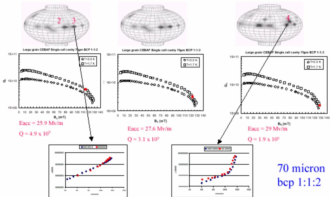
Figure 11: Example of T-maps at different field levels in the Q-drop region of a large grain OC cavity
