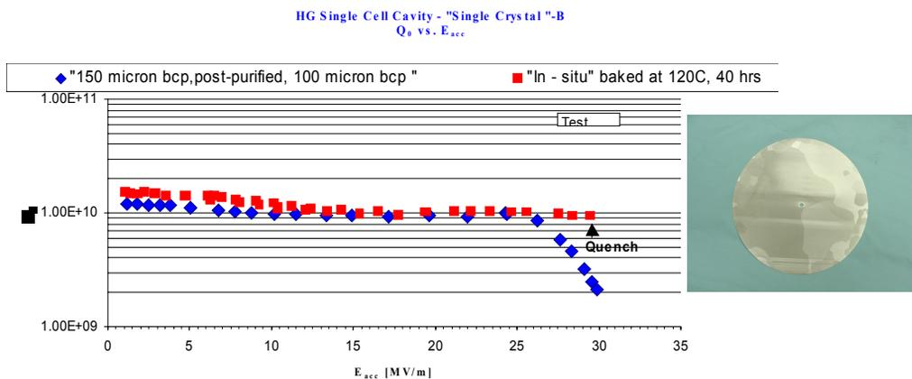
Figure 3: Performance of cavity made from ingot “B”
