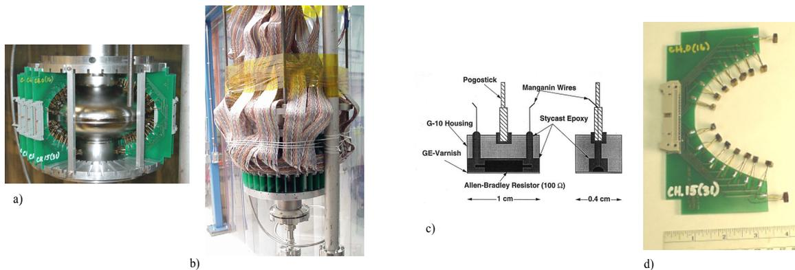
Figure 10: Temperature mapping system, consisting of 36 boards as shown in (c), each equipped with 16 Allen-Bradley carbon resistors (d)
