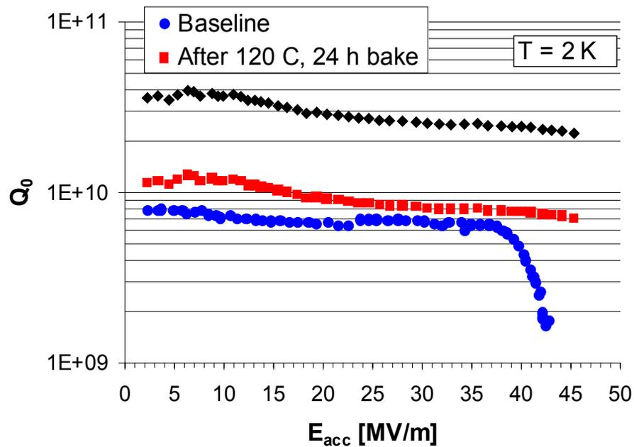
Figure 7: The single crystal low loss cavity as shown in figure 2c [ f = 2.3 GHz, E<sub>peak</sub>/E<sub>acc</sub> = 2.07, H<sub>peak</sub>/E<sub>acc</sub> = 3.56 mT/MV/m] performed very well and quenched at 45 MV/m with a high Q-value after “in situ” baking. The black diamonds in figure 7 are scaled values to a frequency of 1300 MHz.
