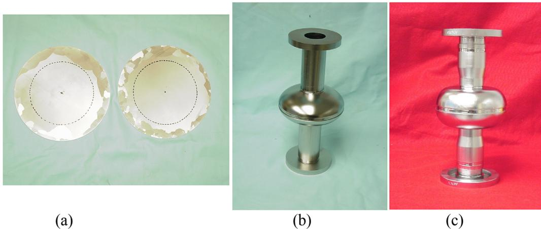
Figure2: Ingot “A” with a large center crystal (a), from which a scaled high gradient (b) and a scaled low loss ( c ) cavity was fabricated.
