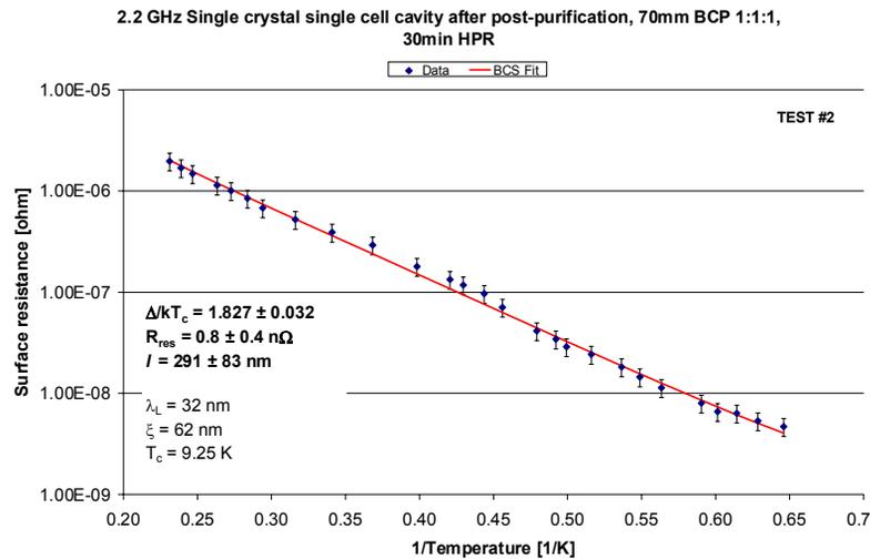
Figure 8: Measured temperature dependence of the single crystal 2.2 GHz cavity [4.2K≤T≤1.6K]
