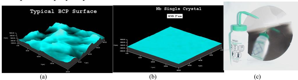
Figure 9: Surface roughness of bcp’d surfaces: (a) typical polycrystalline surface after removal of ~ 100 μm ( roughness 1274 nm), (b) single crystal after 80 μm and mechanical polishing ( roughness 27 nm), for comparison an electropolished poly-crystalline surface had a roughness of 252 nm; (c) reflectivity of bcp’d large grain niobium surface
