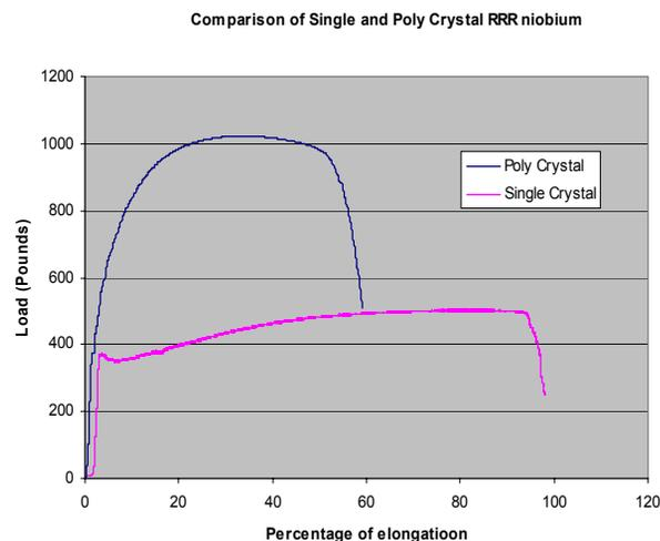
Figure 1: Stress-strain behaviour of single crystal and poly-crystalline niobium
