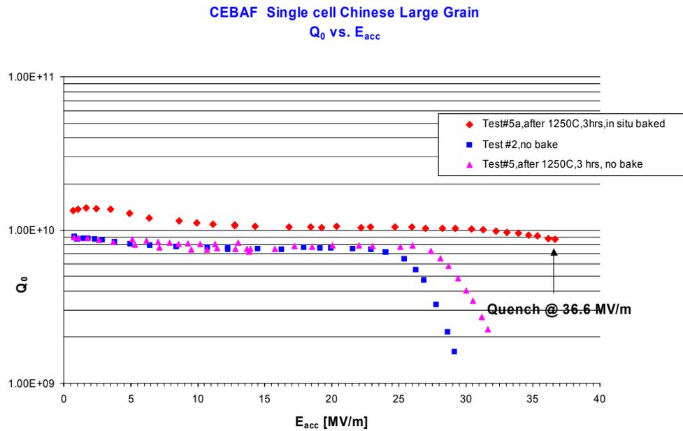
Figure 6: Q vs E<sub>acc</sub> of a single cell OC cavity made from large grain niobium supplied by Ningxia [4]; shown are the performances before and after “in situ” baking. The “quench” field of E<sub>acc</sub> = 36.6 MV/m corresponds to a surface magnetic field of 166 mT.
