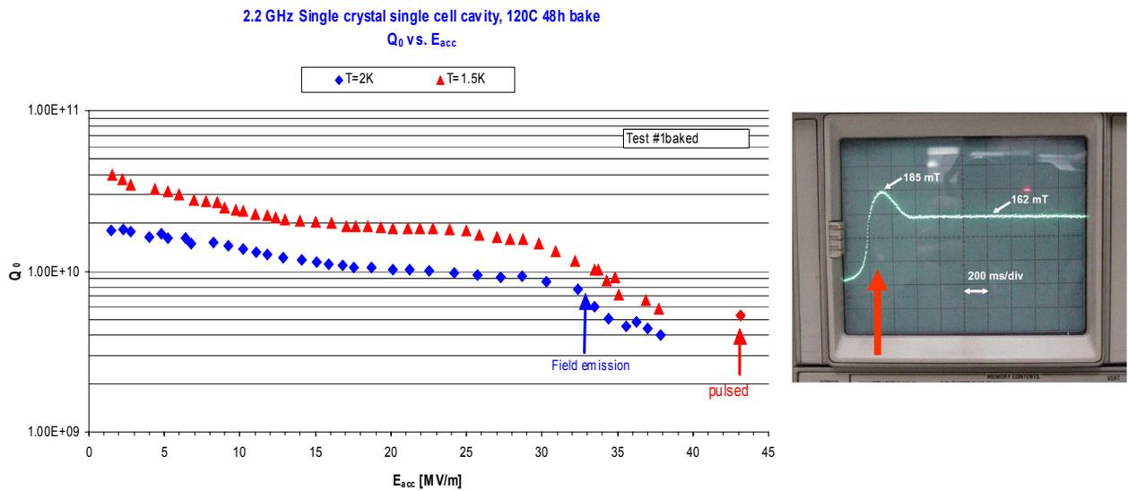
Figure 5: Performance of single crystal HG cavity after 100 micron of material removal by BCP, 800 C hydrogen degassing, add. 100 micron of BCP and “in situ” baking for 48 hrs at 120C; the cavity reached a field of 43 MV/m corresponding to a peak magnetic field of 185 mT under pulse conditions as shown on the oscilloscope trace
