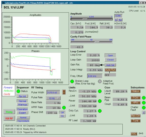
Figure 2. Low Level RF screen showing the RF amplitudes (Forward blue, transmitted red, reflected green) during a quench event for an SNS superconducting cavity. During the quench the loaded Q drops to about  $3 \times 10^5$  and the unloaded  $Q_0$  to  $4 \times 10^5$ .
