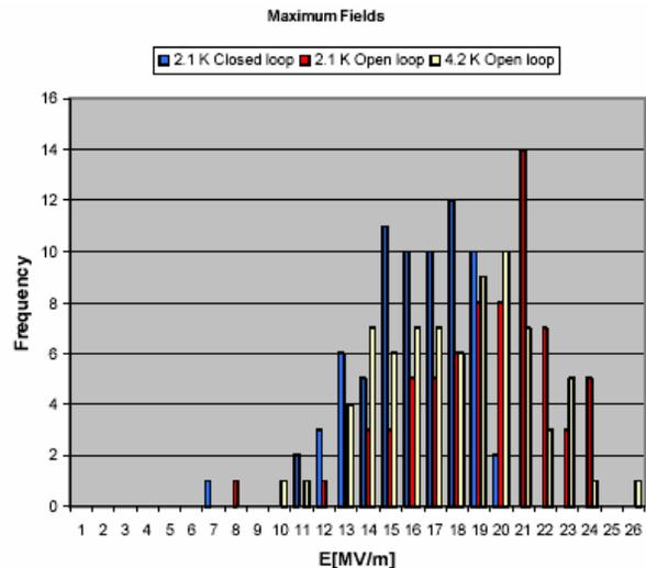
Figure 3. Distribution of maximum gradients achieved in the SNS superconducting cavities so far at 4.2 K in open loop (yellow bars) at 2.1K in open loop (red bars) and at 2.1K in closed loop (blue bars). All data are for 1.3 msec pulse length at 10 pps. The overall average values are 17-18 MV/m.
