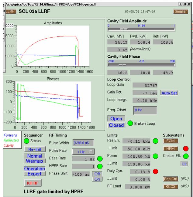
Figure 1. Low Level RF traces of forward (blue) reflected (green) and transmitted (red) amplitude (above) and phase (below) for a SNS superconducting cavity in open loop. Data acquisition terminates 50  $\mu$ sec after the end of the RF pulse
