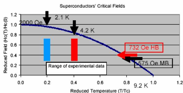
Figure 4. Theoretical magnetic field limits for a superconductor as a function of temperature. The operating values for SNS are well below the theoretical limits (blue curve). Experimental maximum field ranges are essentially identical at 4.2 K (red bar) and at 2.1 K (blue bar).
