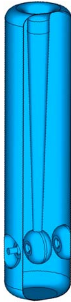
57.5 MHz QWR-based structures .02 < \beta < 0.14
