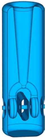
57.5 MHz QWR-based structures .02 < \beta < 0.14
