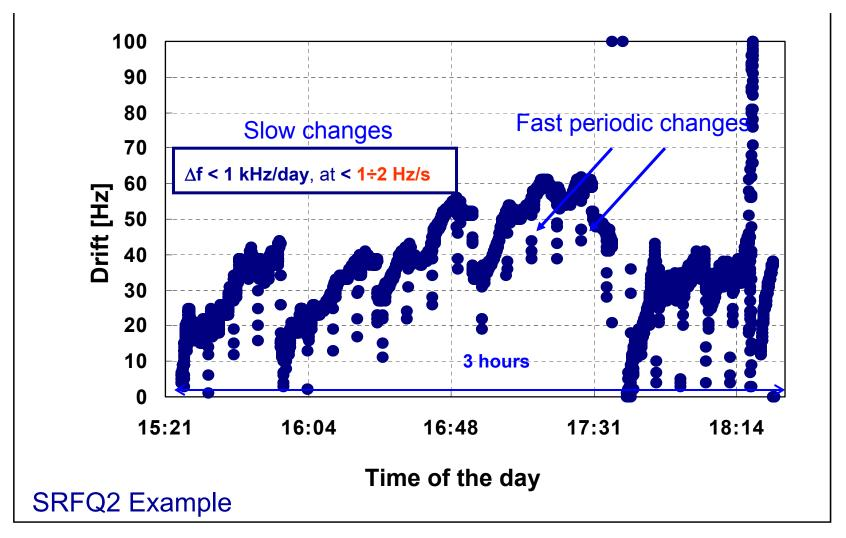
Free f<sub>0</sub> drifts in the test cryostat: slow and fast pressure drifts dominate the scene
