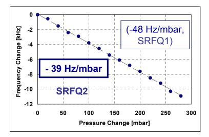
Cryogenic-Plant Specs: 1.2  $\pm$ 0.05 bar;  $\triangle P/\triangle t \le 2 \text{ mbar/min} \rightarrow 1.33 \text{ Hz/s}$
