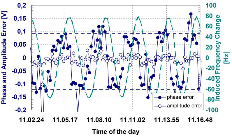
The master oscillator frequency was modulated with sine, square, saw tooth functions of various period and amplitude: the slow tuners follow up to  $\sim 2$  Hz/s (square function case: cavity locked only if  $\triangle f$  is within the bandwidth, i.e. 20 Hz)
