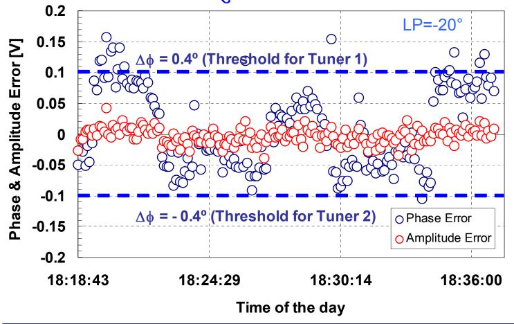
Both SRFQ1 and SRFQ2 could be kept locked, for <u>half-day long tests</u>, <u>beyond 26 MV/m</u>, in the environmental conditions shown previously.
