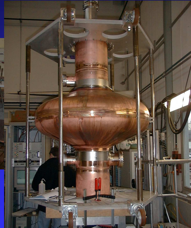
Magnetron Nb film (1-2 \mu\text{m} ) sputtering
